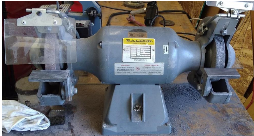
Figure 8.2.2: Polisher Used to Polish Cut Material
