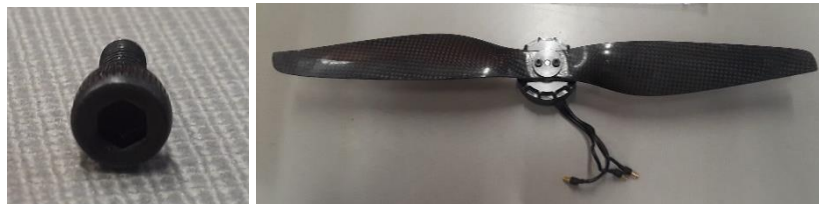
Figure 8.3.20 Propellers attached to motor and socket screw used to do so.
