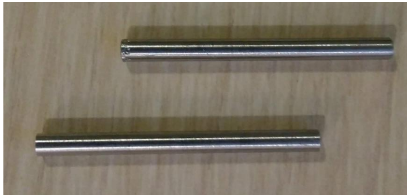
Figure 8.2.3: Pins Used for the Hinge After Being Cut to Size
