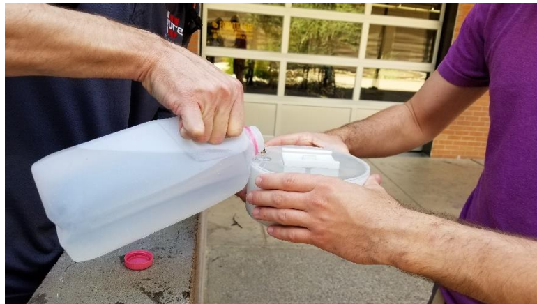
Figure 9.2.3.1.1 Loading of Container with Fluid for Actuation Reliability Test
