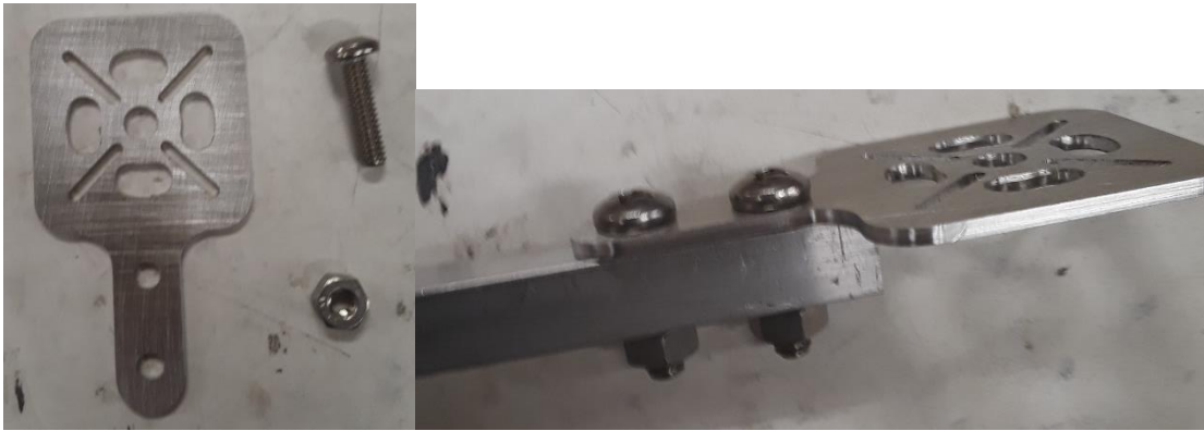
Figure 8.3.13 A motor mount attached to the drone arm with a 1-inch screw with a \frac{1}{4} "- 20 thread and a \frac{1}{4} "-20 thread nut.
