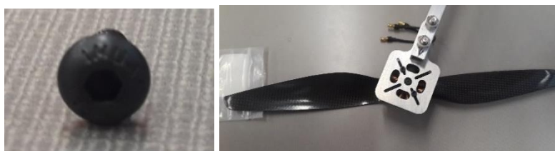
Figure 8.3.21 Motors attached to drone body and capped screws used to do so
