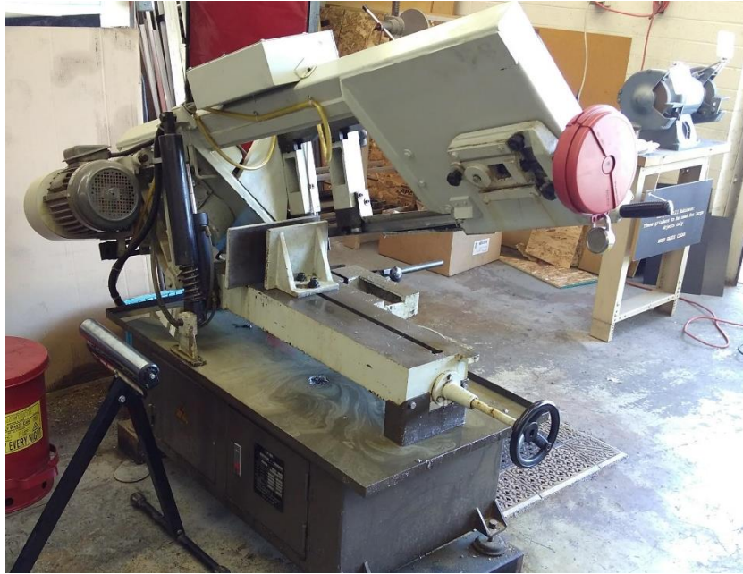
Figure 8.2.6: Band Saw Used to Cut Aluminum Tube
