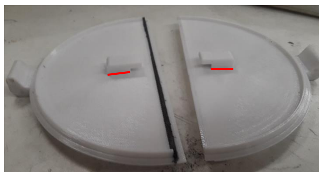
Figure 8.3.6 The lock support bars bonded to the reservoir lid.
