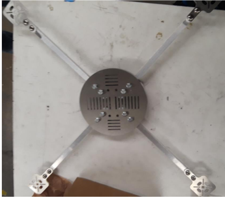
Figure 8.3.15 Complete sub-assembly as the drone base.
