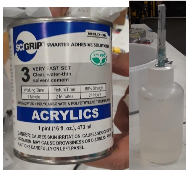
Figure 8.3.5 SciGrip acrylic cement solvent used to bond the plastic pieces together in both its original can and in the drip bottle used for application.
