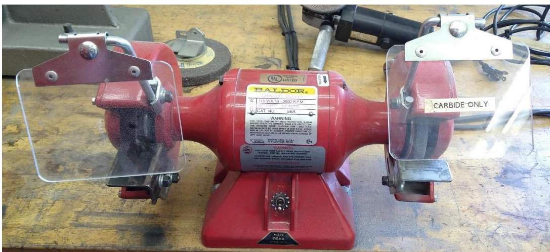
Figure 8.2.1: Grinder Used to Cut Pin to Size
