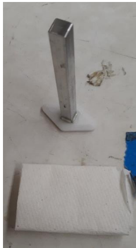
Figure 8.3.4 The actuator pieces joined together along with a small paper towel used to wipe any excess adhesive.
