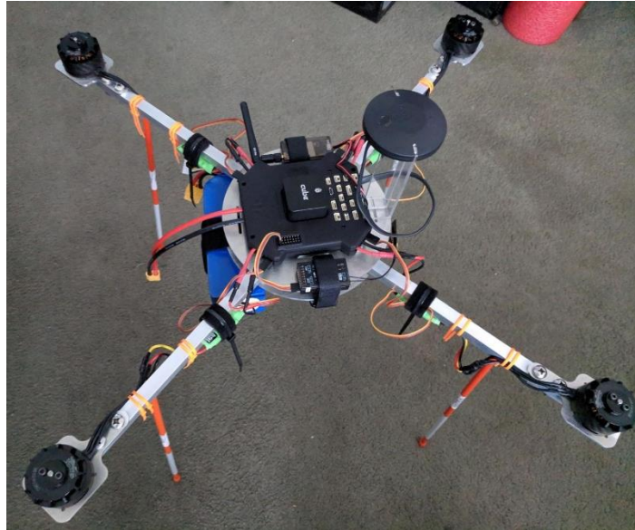
Figure 8.3.22 A photograph displaying the electronics assembly
