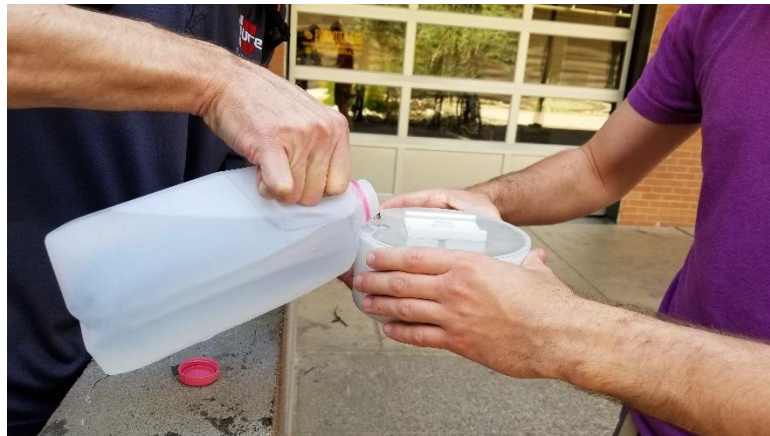
Figure 1: Loading of Container with Fluid for Actuation Reliability Test
