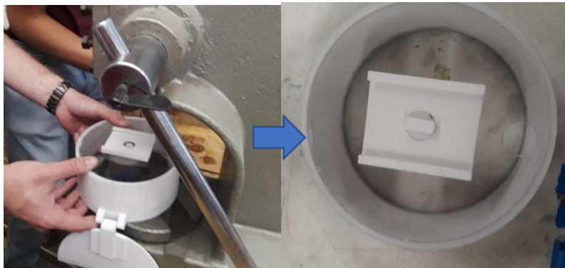
Figure 8.3.16 The reservoir and actuation system being held under the drill press (left) and a top view of the reservoir system after the epoxy dried (right). These photos demonstrate the actuation system assembly process.
