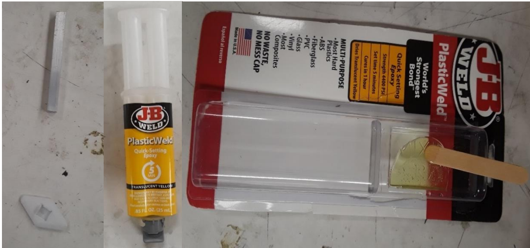
Figure 8.3.3 Actuator rod and locking block along with the JB Plastic Weld epoxy adhesive
