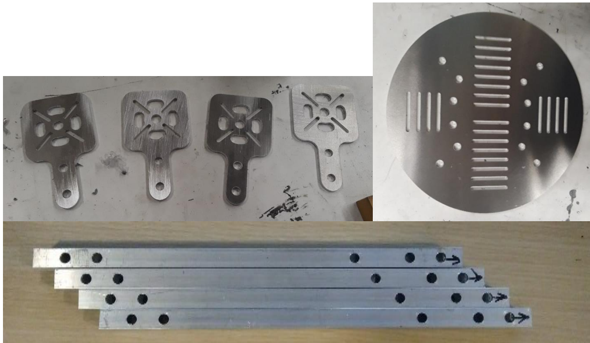
Figure 8.3.11 Parts used for the drone base sub-assembly. Top from left to right: motor mounts and base plates. Bottom: drone arms.
