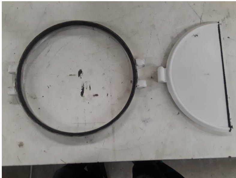
Figure 8.3.2 The chamber parts with sealants adhered.
