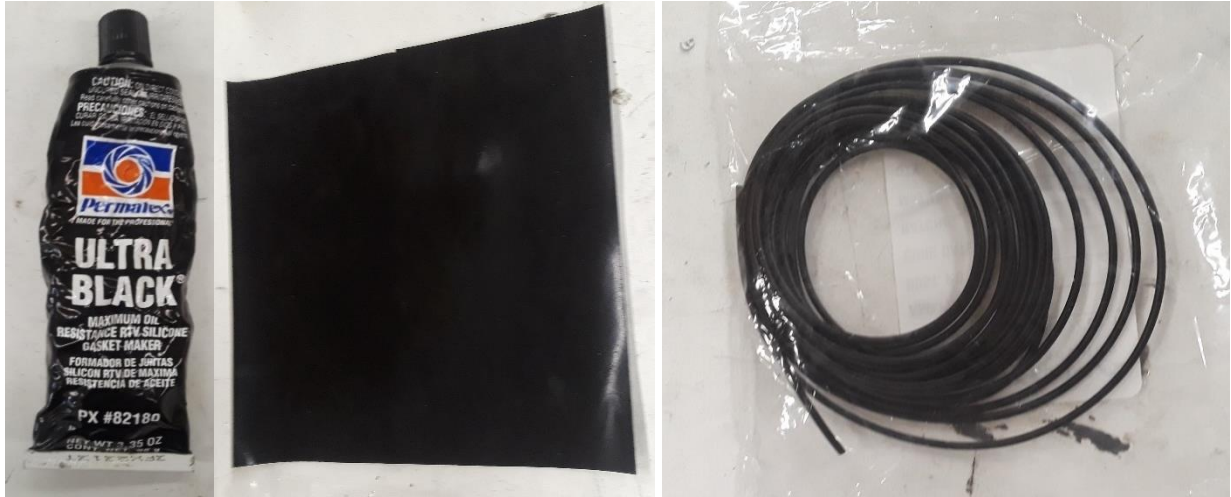
Figure 8.3.1 The materials needed for the gaskets. Pictured from left to right: Ultra Black gasket maker, Buna-N sheet, and U-ring material.
