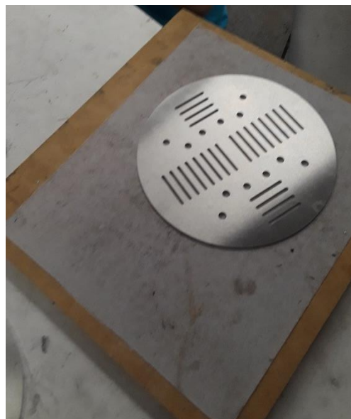
Figure 8.3.12 A plate on the sander used to smooth the freshly cut aluminum.
