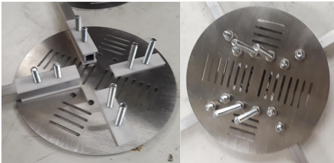
Figure 8.3.14 The base plates of the drone with brackets and arms attached to it with 1\frac{1}{2} inch hex bolts with a \frac{1}{4} "- 20 thread and the same \frac{1}{4} "-20 thread nut used on the motor mounts.
